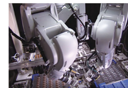
Assembly work that maintains the relative positions for mutual gripping
