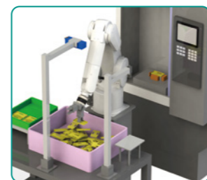
Picking from a large pallet (Fixed camera)
