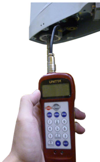
Fig.5-7 : Tension adjustment method of timing belt
