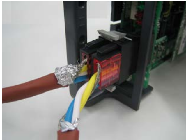
Figure 6.2-2 The example of one-touch connector connection for two or more station connection
