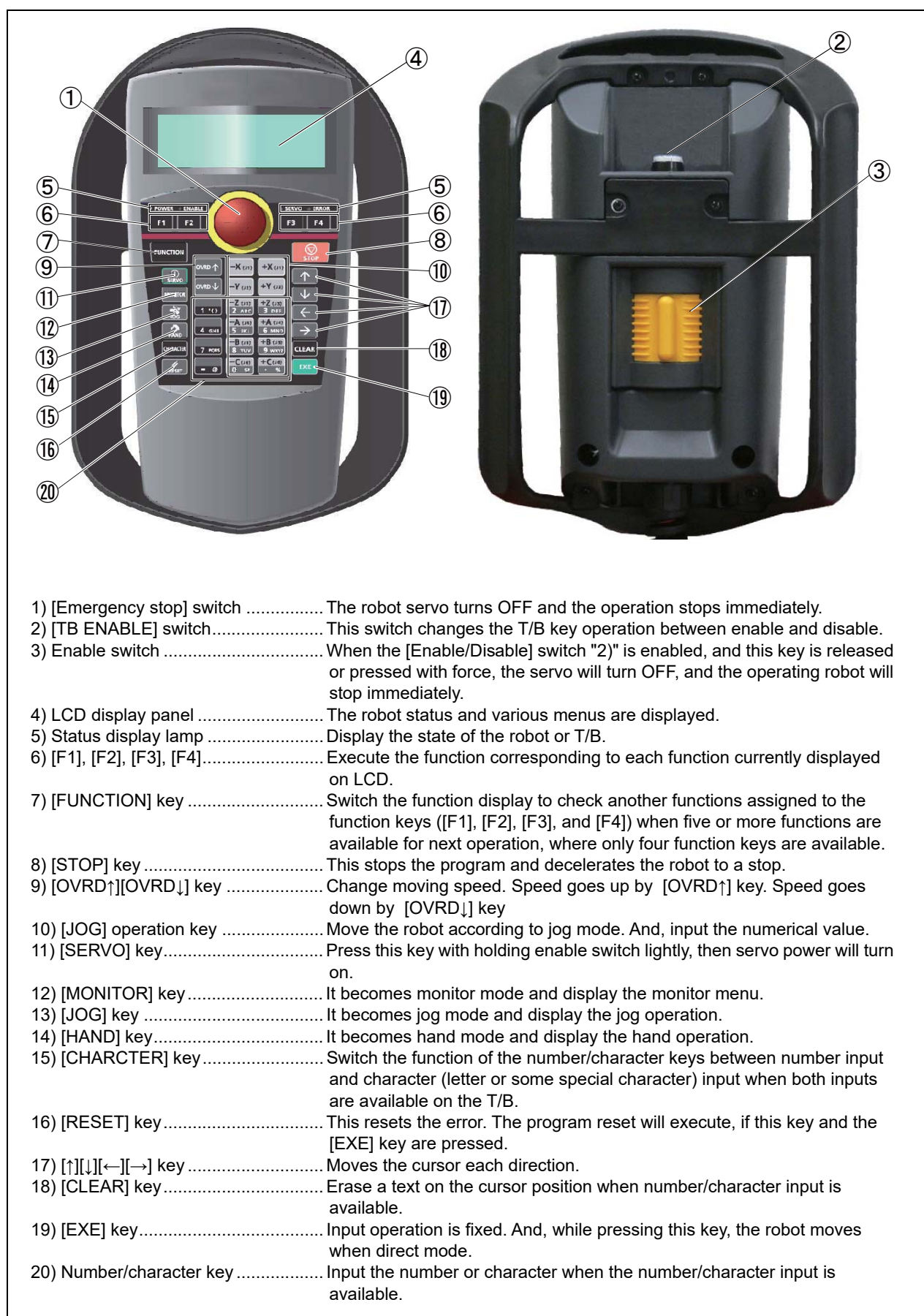
Fig.3-19: Teaching pendant key layout and main functions
