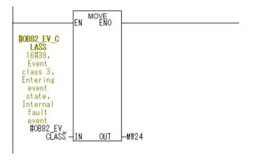
The data type of the error detection data is converted. Conversion (byte to int)
