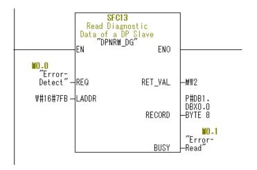
"Diagnostic Data" is transmitted to DB1 when the error detection is ON.
