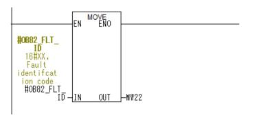
The data type of the error code is converted.
