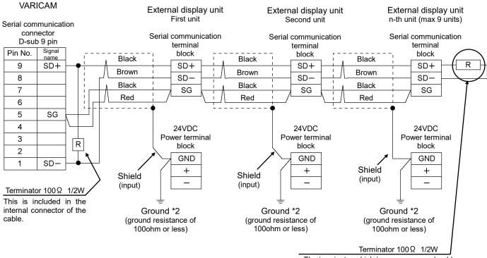
The terminator which is an accessory should be installed at the last external display unit.
