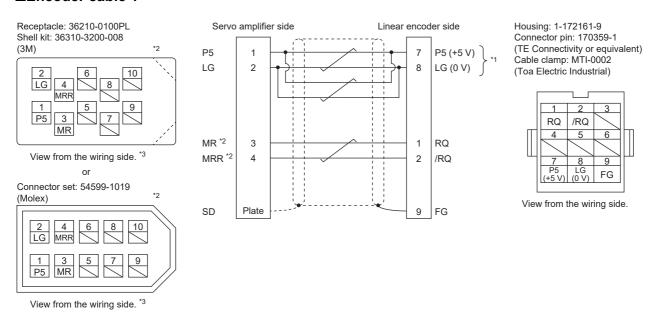
\*1 Encoder cables that meet the following specifications are recommended.
