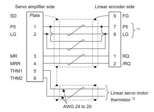
Housing: 1-172161-9 Connector pin: 170359-1 (TE Connectivity or equivalent) Cable clamp: MTI-0002 (Toa Electric Industrial)
