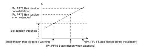
Belt tension threshold = [Pr. PF76 Belt tension irregular threshold]/100 × [Pr. PF72 Belt tension on installation]
