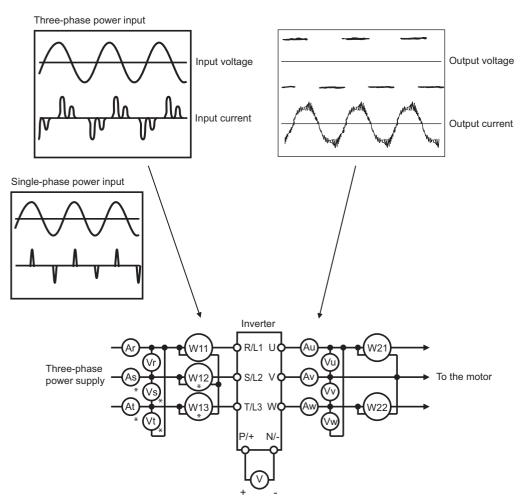
\* At, As, Vt, Vs, W12, W13 are only for the three-phase power input specification models.
