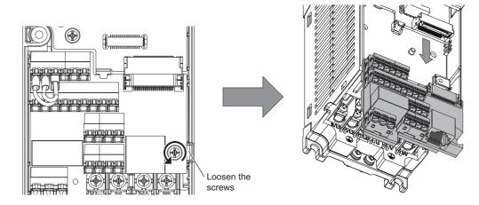
**2.** Be careful not to bend the pins of the inverter's control circuit connector, reinstall the control circuit terminal block and fix it with the mounting screws.
