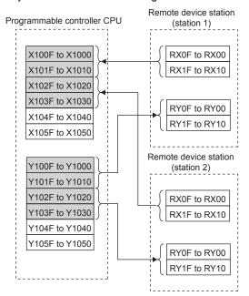
• The relation between the device of the programmable controller CPU and remote register (RWw, RWr) of the remote device station is as follows: The devices used actually are indicated in shaded regions.
