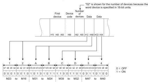
When word devices are used, one word is specified in 16 bits as follows. The data is stored from the lower byte (bit 0 to bit 7) to the upper byte (bit 8 to bit 15).
