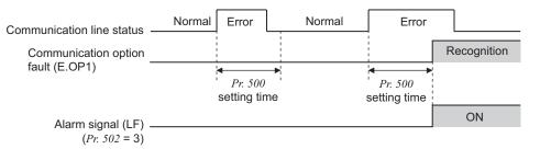
When a communication line error occurs and lasts longer than the time set in *Pr. 500*, it is recognized as a communication option fault.
