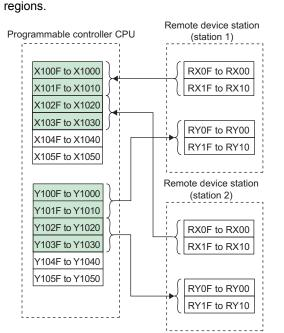
(4) The relation between the device of the programmable controller CPU and remote register (RWw, RWr) of the remote device station is as follows:
