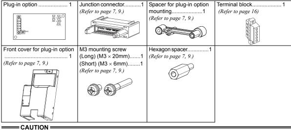
• Install a provided front cover for plug-in option, in place of the inverter front cover .
