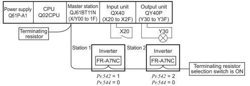
(2) Network parameter setting of the master station Network parameters are set as below.
