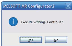
8. Writing of the servo parameters is started and all the parameters are written to the servo amplifier.
