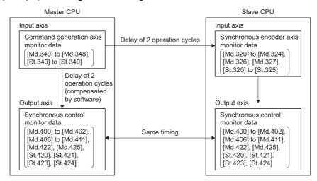
• To remove the delay time described above, using the phase compensation function of the output axis for the slave CPU and the master CPU, set a value that adds a delay compensation time of two operation cycles to the delay time inherent to the system. Refer to phase compensation on delay time of the input axis for delay time inherent to the system. (Fig. Page 163 Phase compensation on delay time of the input axis)
