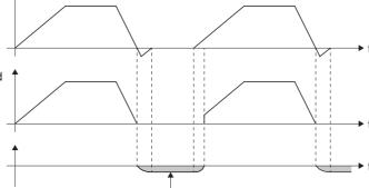
The input travel value is accumulated as a rotation direction restricted amount, and will be reflected when the input travel value moves in the enable direction.
