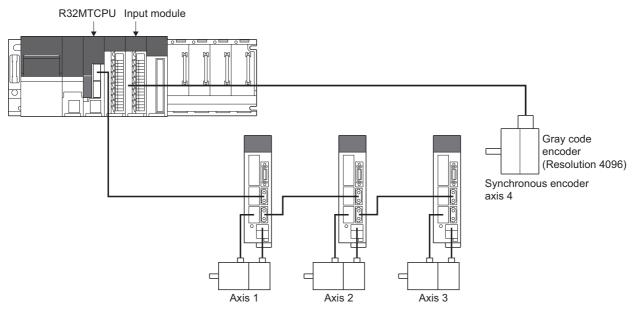
Set the following in Synchronous encoder axis setting Resolution of synchronous encoder via device of synchronous encoder axis 4 on the synchronous encoder axis parameter screen of MT Developer2.
