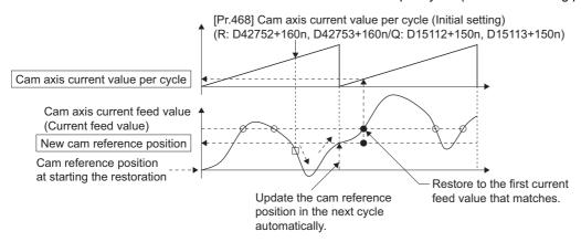
Search from a value in the middle of the cam axis current value per cycle. (Cam data starting point ≠ 0)
