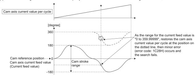
• In the case above, execute cam axis current value per cycle resoration within a cam stroke range exceeding 0 and less than 360[degree]
