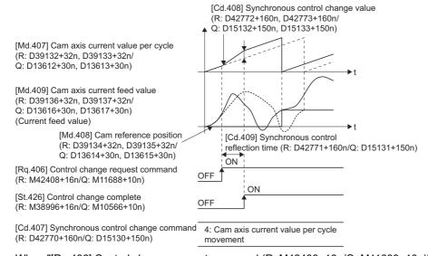
When "[Rq.406] Control change request command (R: M42408+16n/Q: M11688+10n)" is reset to OFF while executing the cam axis current value per cycle movement, operation is stopped midway. If the cam axis current value per cycle movement is executed again, the remainder travel value is not reflected, and the operation starts with "[Cd.408] Synchronous control change value (R: D42772+160n, D42773+160n/Q: D15132+150n, D15133+150n)" to be used again.
