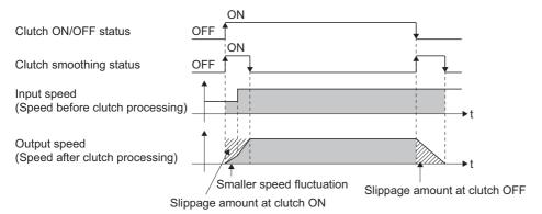
• When "5: Slippage method (Linear: Input value follow up)" is set The output speed fluctuates with the input speed. (When re-accelerating after the input speed is dropped, a sudden acceleration may occur)
