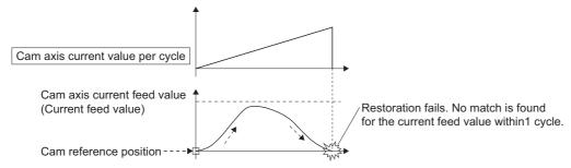
(2) When the unit is "degree" and cam axis current value per cycle restoration is executed in a cam stroke range that straddles 0
