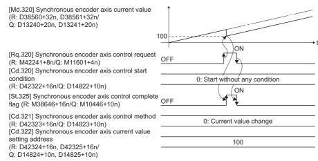
When this signal is ON, if "101 to 164" is set to "[Cd.320] Synchronous encoder axis control start condition (R: D42322+16n/Q: D14822+10n)", the synchronous encoder axis control starts based on the corresponding high-speed input request signal.
