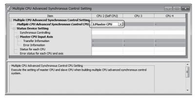
Set the master CPU servo input axis settings in the servo input axis parameters. ( Fage 32 Servo input axis parameters)
