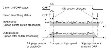
• When "5: Slippage method (Linear: Input value follow up)" is set The clutch smoothing status ON section is fixed.
