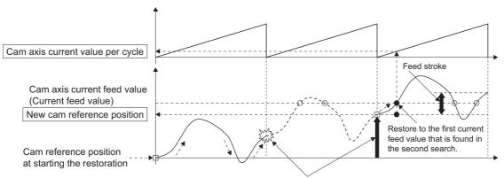
Once the restoration fails in the first search, the new cam reference position is automatically updated to the one within the feed stroke amount, which is equal to "Current feed value - New cam reference position", and the search process starts again.
