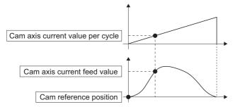
Select from 3 objects as follows in "[Pr.462] Cam axis position restoration object (R: D42742+160n/Q: D15102+150n)" which position is to be restored. ( Page 148 Cam Axis Position Restoration Method)
