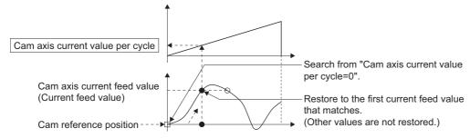
• Search from a value in the middle of the cam axis current value per cycle. (Cam data starting point = 0)
