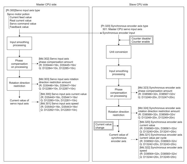
• If "501: Master CPU synchronous encoder axis" in "[Pr.320] Synchronous encoder axis type" is selected.
