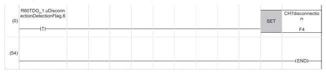
(0) At the time when disconnection is detected in CH7, the processing is to be performed.
