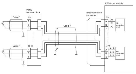
\*1 Use a shielded cable and ground the shields.
