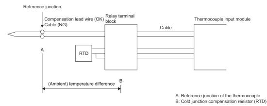
Case 2 (a compensation lead wire is connected between the relay terminal block and the thermocouple input module)
