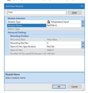
4. Configure the setting to use the module labels and add the module labels of the temperature input module.
