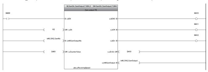
**5.** Reflect the cam output status set by the cam output FB to Y device to refresh it.
