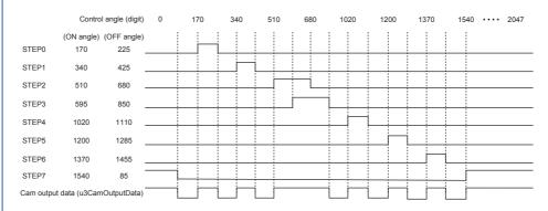
When the cam output data is not set, the ON angle and OFF angle of STEP 0 to STEP 7 become 0. To prevent the ON output without setting, when the ON angle and OFF angle are the same in a STEP, the corresponding angle outputs OFF.
