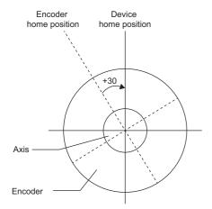
An absolute encoder resolution of 2048 is converted so as to be treated as  $360^{\circ}$  in the program for easy-to-understand control angles, and the Y devices are controlled as follows.
