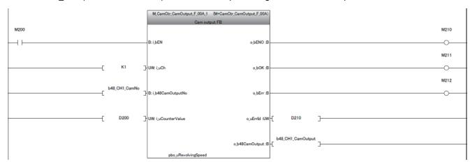
7. Reflect the cam output status set by the cam output FB to Y device to refresh it.
