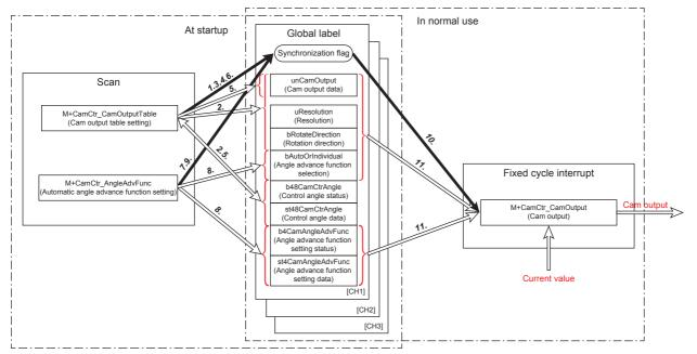
At the startup, use M+CamCtr\_CamOutputTable (Cam output table setting) and M+CamCtr\_AngleAdvFunc (Automatic angle advance function setting) and set each cam output data of the global label.
