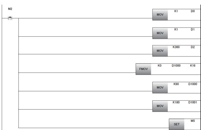
**4.** Set the cam output table by turning on i\_bEN (Execution command).
