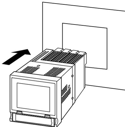
(2) Remove the sheets covering the mounting bracket holes. Fix two mounting brackets either on the sides or on the top and bottom of the unit. Tighten screws.
