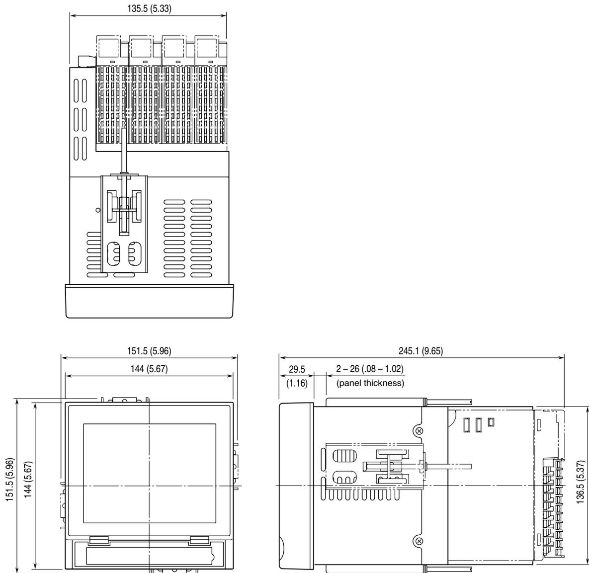
Attach the mounting bracket either on the top/bottom or on the sides.
