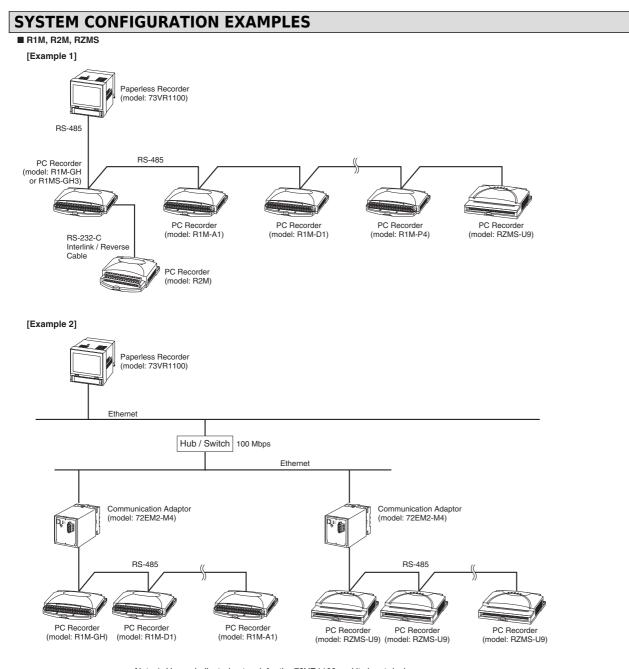
Note 1: Use a dedicated network for the 73VR1100 and its input devices. Note 2: The sampling rate depends upon the number of devices to be connected.
