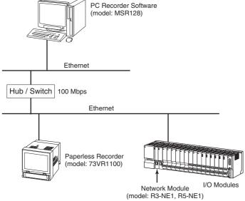
Note 1: Use a dedicated network for the 73VR1100 and its input devices. Note 2: Use of a hub/switch via straight cables is recommended to connect the 73VR1100 to the PC. Note 3: The storing intervals of 100 msec. and 200 msec. are not applicable to the above configuration.
