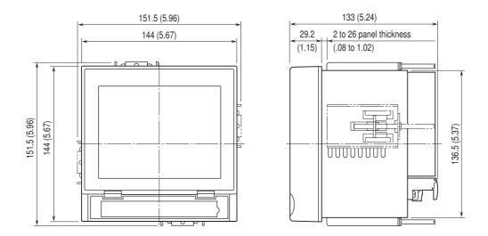
Attach the mounting bracket either on the top/bottom or on the sides.
