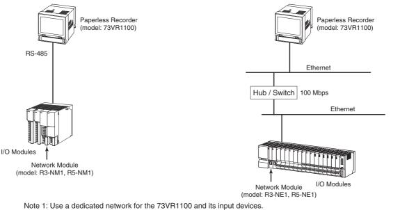
Note 1: Use a dedicated network for the 73VR1100 and its input devices. Note 2: The sampling rate depends upon the number of devices to be connected for the R3 series. Note 3: Use of a switch/hub via straight type cables is recommended to connect the R3-NE1 or the R5-NE1 to the 73VR1100.
