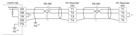
\*1. Internal terminating resistor is used when the device is at the extreme end of a transmission line.
