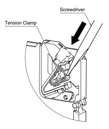
2) Insert a wire. Push the screwdriver toward the direction indicated with the arrow in the figure below to widen the opening if necessary.
