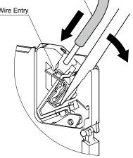
3) Confirm that the wire tip hits the bottom and pull out the screwdriver in holding it in position.
