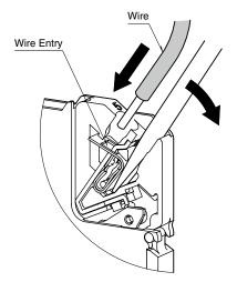
3) Confirm that the wire tip hits the bottom and pull out the screwdriver in holding it in position.
