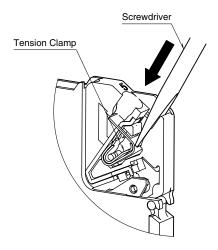
Insert a wire. Push the screwdriver toward the direction indicated with the arrow in the figure below to widen the opening if necessary.
