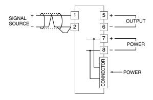
The M6SVF, by its fast-response feature, is not designed to eliminate noise present in the input signal. Use a shielded twisted-pair cable to prevent noise from entering through the input wiring.
