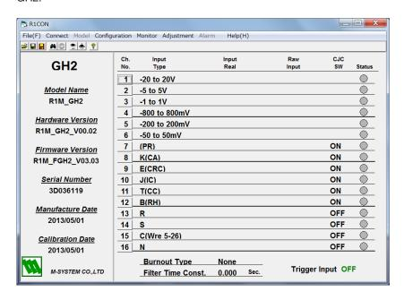
With the R1C-GH2's firmware version V1.xx, the model name may be indicated as 'R1M,' though the programming is performed correctly.
