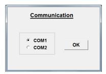
Confirm that the power is supplied to the R1x and that the configurator jack of the R1x and the COM1 port of the PC is firmly connected with the attached cable.
