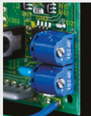
Multi-turn potentiometer for fine adjustment
