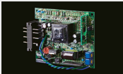
Multi-turn potentiometer for fine adjustment
