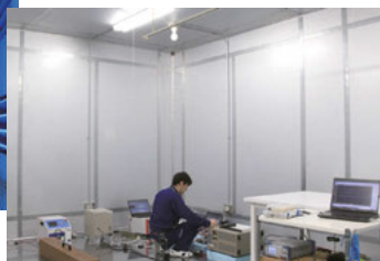
Anechoic chamber certified and registered by the official body (VCCI (5) )
