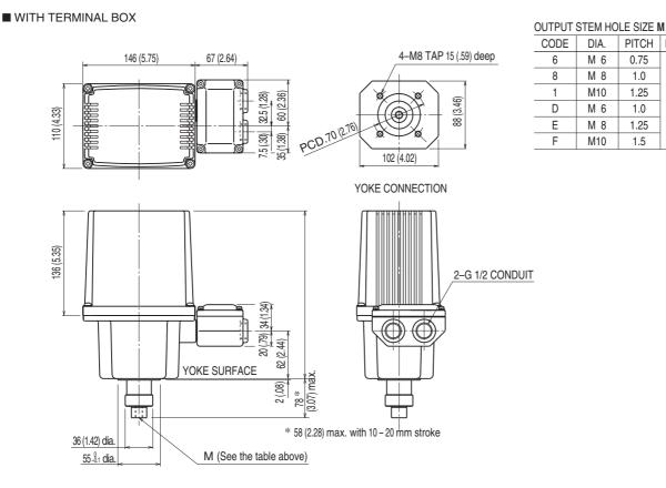
Cable connector or leadwires not provided with terminal box.
