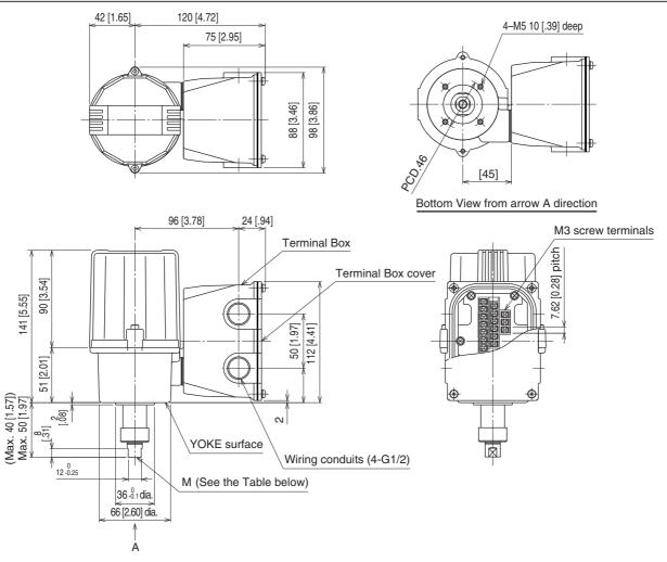
The dimension in ( ) is when the stroke is set to 5 to 10 mm.
