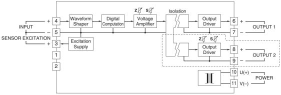
Note 1: The section enclosed by broken line is only with 2nd output option.
