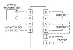
The section enclosed by broken line is only with 2nd output option. DO NOT connect to the terminal 1.
