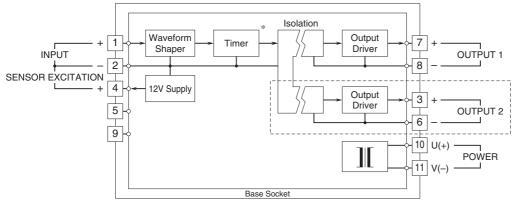
\*The timer is provided when the low frequency open collector or the dry contact AC/DC switch is selected as one of the outputs.
