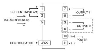
The section enclosed by broken line is only with 2nd output option
