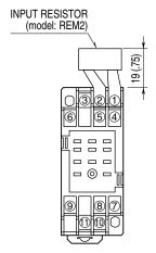
Input shunt resistor attached for current input.
