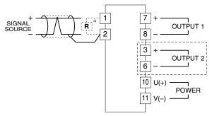
\*Input shunt resistor attached for current input.
