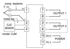
The section enclosed by broken line is only with 2nd output option.
