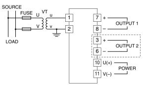
The section enclosed by broken line is only with 2nd output option.
