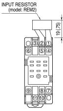
Input shunt resistor attached for current input.
