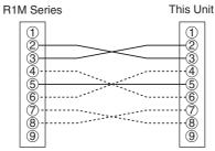
The above connection including solid and broken lines is an example of 'Interlink' cable.
