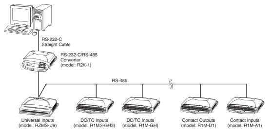
When the cable distance between the PC and the I/O modules is long, insert an RS-232-C/RS-485 Converter for isolation.
