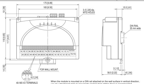
use of a attachment plate to prevent the module from sliding down is recommended.
