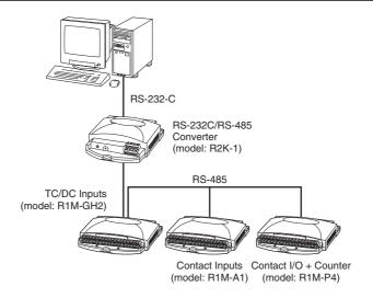
When the cable distance between the PC and the R1Ms is long, insert an RS-232-C/RS-485 Converter for isolation.
