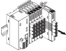
• Removing an intermediate module
