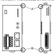
Confirm that the locking clamps of the extension power supply module are set. Insert the module in parallel to the next one while aligning the grooves of both modules (A & B in the above figure). Maintain it perpendicularly to the rail.
