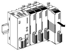
• Removing an intermediate module
