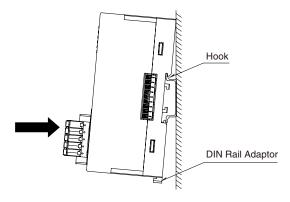
Position the upper hook at the rear on the DIN rail and push in the lower. When removing the module, push down the DIN rail adaptor utilizing a flat-blade screwdriver and pull.
