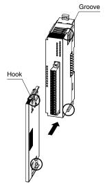
The protective cover is to be attached over the connected I/O module at the right end.
