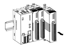
• Removing an intermediate module
