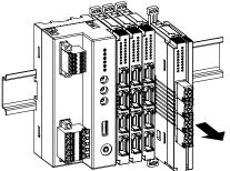
• Removing an intermediate module
