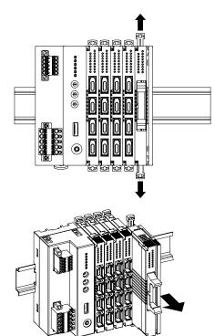
Removing an intermediate module
