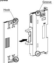
The protective cover is to be attached over the connected  $\ensuremath{\mathsf{I/O}}$  module at the right end.
