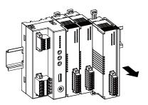
• Removing an intermediate module
