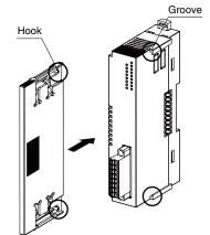
The protective cover is to be attached over the connected I/O module at the right end.
