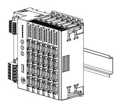
When removing the cover, pull it out while squeezing the hooks inward.
