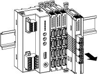
• Removing an intermediate module
