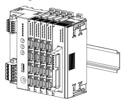
When removing the cover, pull it out while squeezing the hooks inward.
