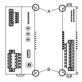
Confirm that the locking clamps of the I/O module are set. Insert the module in parallel to the next one while aligning the grooves of both modules (A & B in the above figure).
