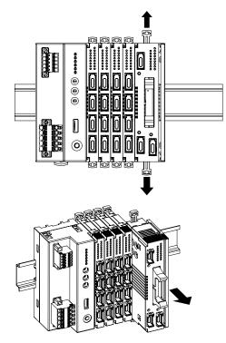
• Removing an intermediate module
