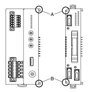
Confirm that the locking clamps of the I/O module are set. Insert the module in parallel to the next one while aligning the grooves of both modules (A & B in the above figure). Maintain it perpendicularly to the rail.
