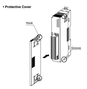
The protective cover is to be attached over the connected I/O module at the right end.
